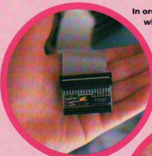
PortPlus Jr is easy to fit to the set of expansion pins on the A1200's motherboard, and provides a speedy extra serial port.
