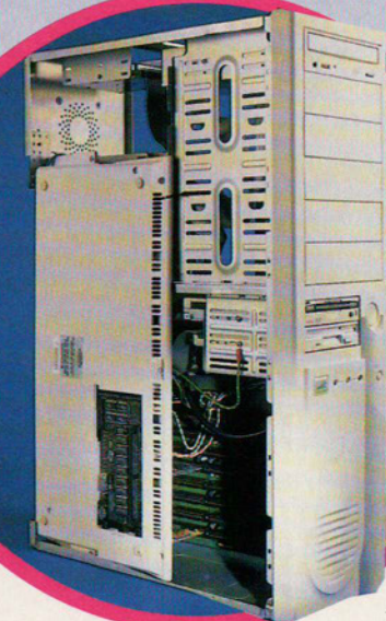
The Eyetech Tower uses a specially modified case which allows an A1200 to be fitted easily and securely. This is definitely one of the easiest solutions to building your own computer.
